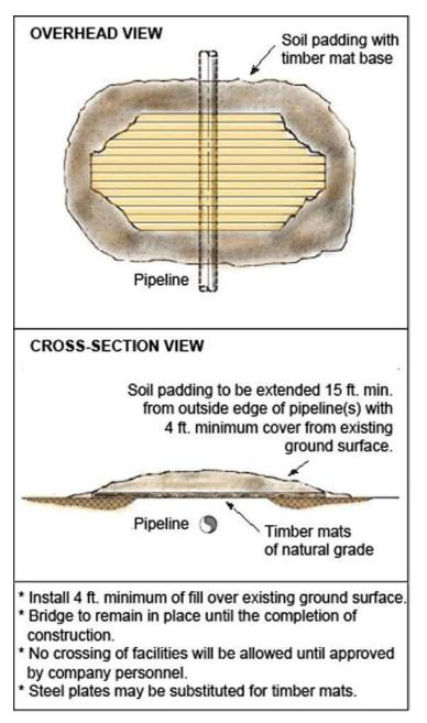
FIGURE 8: REQUIREMENTS FOR HEAVY EQUIPMENT CROSSING A PIPELINE.
