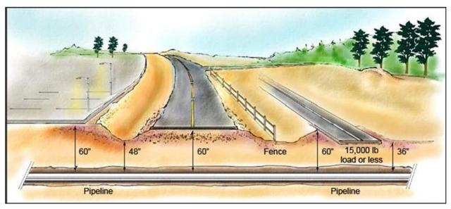
FIGURE 4: ALL ROADS, PARKING LOTS, DRIVEWAYS, AND HEAVY EQUIPMENT CROSSINGS MUST BE APPROVED PRIOR TO INSTALLATION. SEE SAMPLE BELOW.
